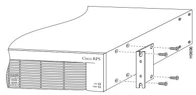
Note: The second bracket attaches to the other side of the chassis.
